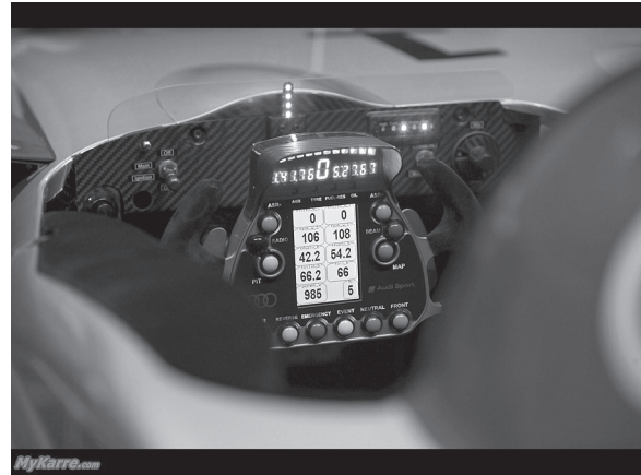
Figure 9 Cockpit display unite made by using Embedded Technology PCBs based on the AML technology developed by Hofmann Leiterplatten in Germany. Excellent readability, light weight and well protected against shock and pollution are key factors for this construction.
