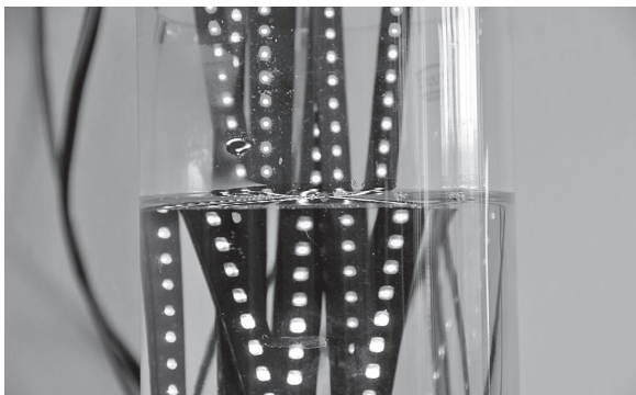
Figure 8 shows an example how PCB technology supports the embedding of LEDs to improve long term performance. In this example the assembled PCBs with LEDs are placed in water for more then 4 years and have still a useful life
